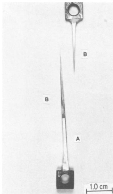
**Figure 5** Needle-point fracture in the beta phase. No visible plastic deformation in alpha in a specimen tested at  $538^\circ \text{C}$  with a crosshead speed of  $0.10 \text{ cm min}^{-1}$ . Yield stress of beta  $10.8 \text{ MN m}^{-2}$ . Critical resolved shear stress of beta  $5.1 \text{ MN m}^{-2}$ . Total strain 150%.
