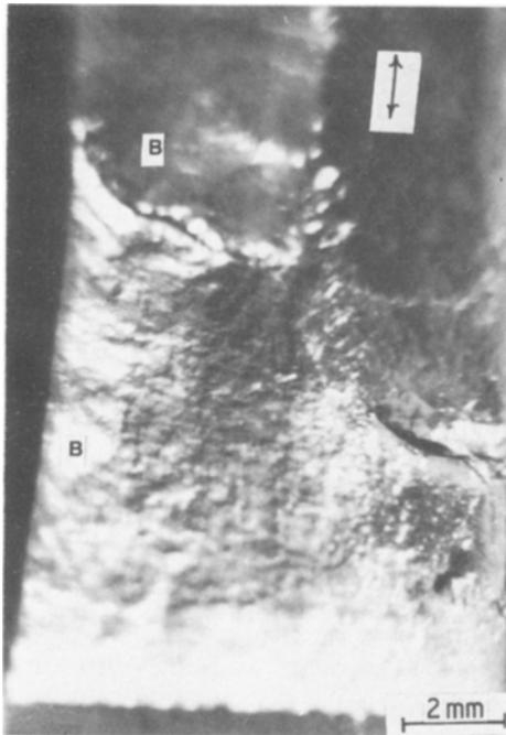
*Figure 2* Severe deformation in the beta region near the phase boundary in a specimen tested at 482° C with a crosshead speed of 0.10 cm min<sup>-1</sup>. Yield stress of beta 16.9 MN m<sup>-2</sup>. Critical resolved shear stress of beta 8.33 MN m<sup>-2</sup>. Total strain 12.56%.
