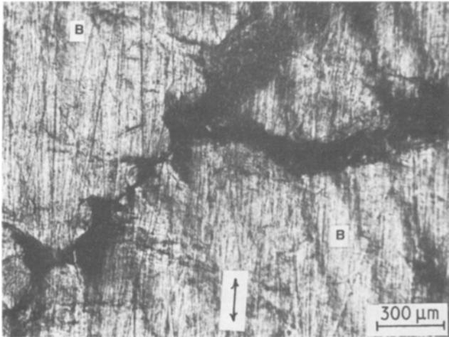
*Figure 1* Severe deformation and grain boundary cracking in the beta phase away from the phase boundary in a specimen deformed at 482° C with a crosshead speed of 0.02 cm min<sup>-1</sup>. Yield stress of beta 9.5 MN m<sup>-2</sup>. Critical resolved shear stress of beta 4.7 MN m<sup>-2</sup>.
