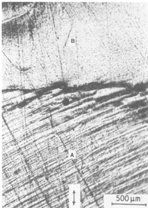
**Figure 4** Interaction of single slip in alpha with the boundary. Deformation in alpha has progressed through the boundary into beta regions. Crosshead speed  $0.5 \text{ cm min}^{-1}$ .
